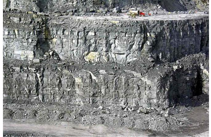
The customer challenge was to provide more consistent rock breakage and displacement from the blasts along with reducing the ground vibration readings. The implementation of more accurate and more precise delay timing ensured overall production costs remained level. Providing consistent rock fragmentation and muck displacement reduces pit operations cost balanced even with the additional cost associated with advanced initiation systems.
