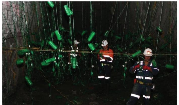
*Loading electronic detonators in production charging.*
