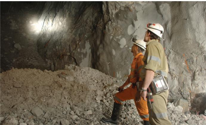
Personnel conducting an inspection of a fired stope.
