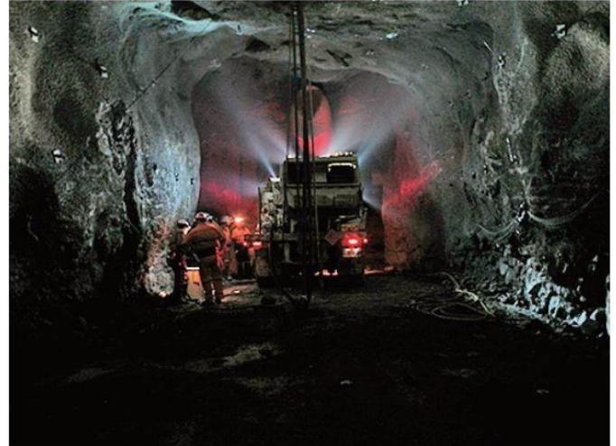
The mining method employed at the site is Panel Caving which is a natural caving method that uses ground stresses, rock structures and gravity to break the rock. The Cadia East mine is the first panel cave in Australia and the deepest panel cave in the world with the extraction level lying approximately 1,200m below the ground surface. Ore is extracted using a mechanised fleet and delivered to the surface through an underground conveying system for processing.
