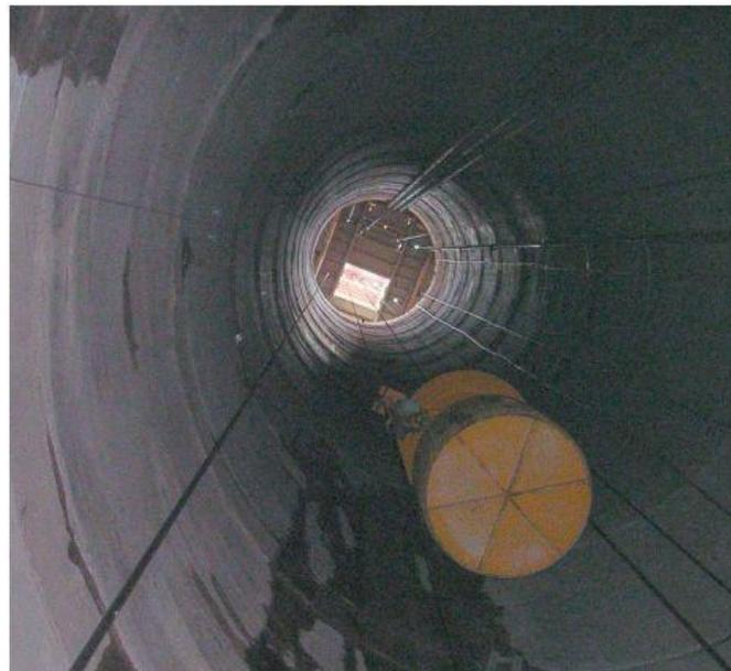
All production holes were charged with bulk emulsion using a cartridge primer.
