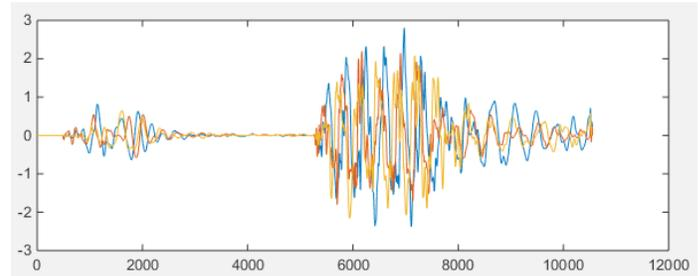
The PPV from the cast that was shot with the signature hole was 1.24 IPS at the well. The distance from the well was 2,000 feet. The delay timing sequence was chosen by DynoConsult.
