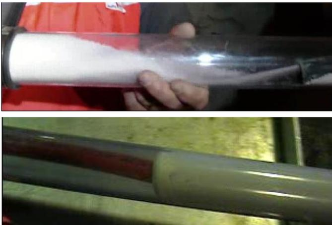
**Figure 2: ANFO hose (Top) and Titan 7000 hose (bottom)**
