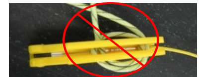
Incorrect connection > Cord not in centre groove
