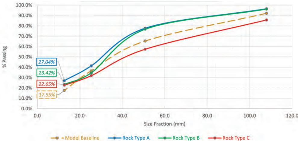
Figure 3. Drill to Mill optimised blast results vs. baseline weighted average PSD by rock type.
