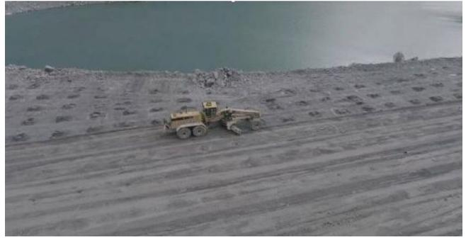
*A grader smooths over a preloaded WebGen 200 Wireless bench to be used as a haul road until blast date. Photo: Orica*
