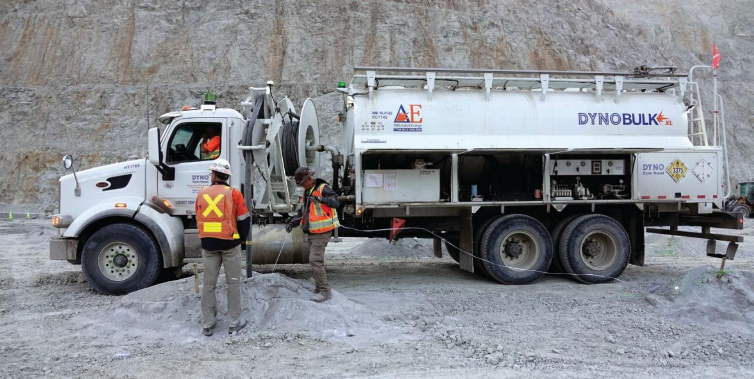
*Dyno Nobel's DIFFERENTIAL ENERGY2 (ΔE2) allows operations to customize the explosive load in individual boreholes based on the unique geological features encountered during drilling. Photo: Dyno Nobel*
