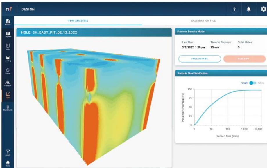
At Dyno Nobel, we've developed a new method that uses a signature waveform approach with a much higher degree of accuracy and confidence. We create a calibrated vibration model based on a previous production blast result, synthetically recreating a known outcome stochastically to account for those previously elusive variabilities that are inherent in blasting.
