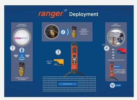
Dyno Nobel's Ranger system, having a potential application in small-scale mines, comes with a flexible tagging option that allows the user to assign both hole location and delay time at the hole or assign delay times at any time the user prefers
