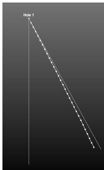
the hole may be as much as 10 feet more than designed. The Boretrak probe was lowered to the bottom of the hole and a reading was taken every 2 meters as the probe was pulled up the hole. The data collector recorded the position of the probe, depth, angle, and azimuth of the hole.
