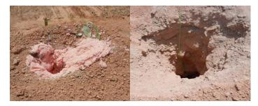
Figure 2 (L-R) Heavy ANFO after loading vs.  $\varDelta E$  after loading
