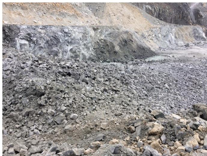
The bench was laid out using a 3D laser profiler and it was determined that 20° holes would be necessary on the first row. The front row was backed up by a row of 10° holes, then a third row of vertical holes. A Boretrack survey was done on the 20° holes and they were found to be within 1° accuracy. The delay design was developed using Signature Hole Analysis and DigiShot<sup>®</sup> electronic detonators. In addition, the initiating hole was deck delayed to minimize the air-overpressure.
