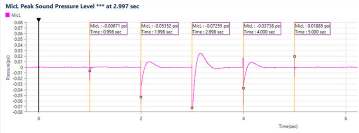
Seismograph data showing the sound produced from shooting 5 detonators sequentially. Each detonator triggered within the target of 1000 ms.
