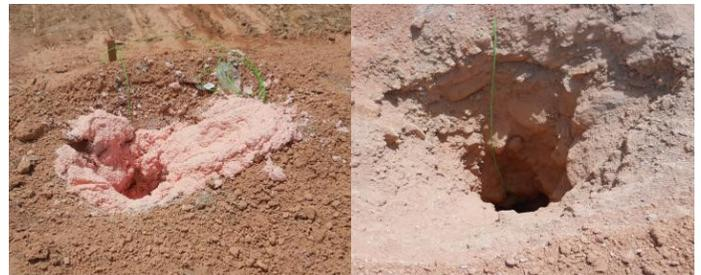
Figure 2 (L-R) Heavy ANFO after loading vs.  $\Delta$ E after loading
