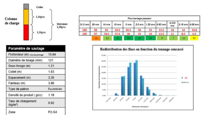
Figure 2: Parameters for blast no. 2014-12
