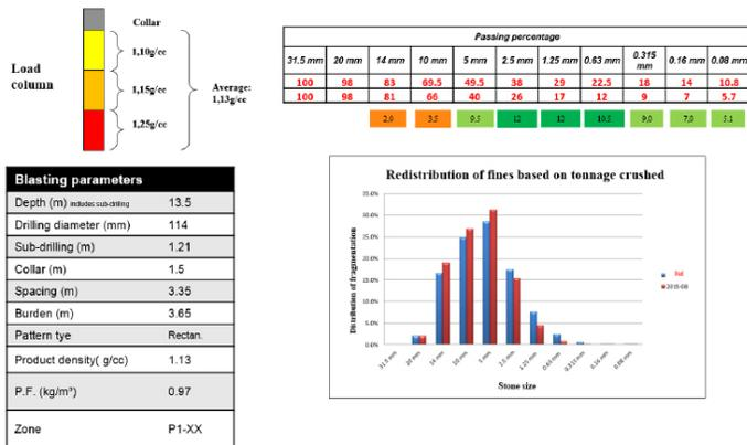
Figure 3: Parameters for blast no. 2015-08
