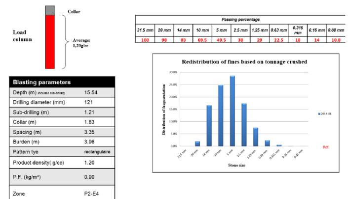
Figure 1: Parameters for blast no. 2014-08
