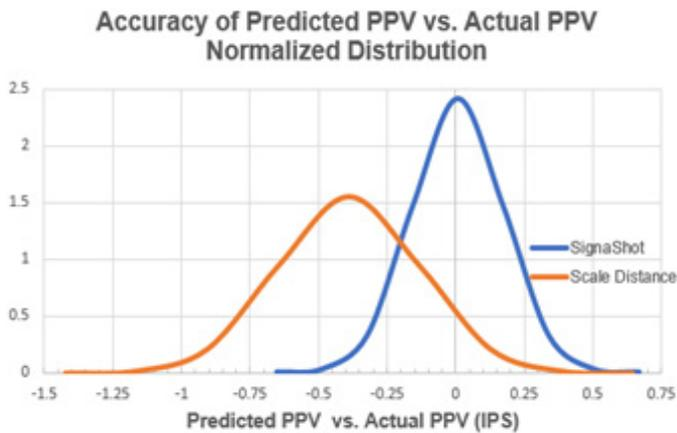
*SignaShot Predictions Outperformed Scale Distance with a Mean Difference of ~0 IPS and Lower Deviation*
