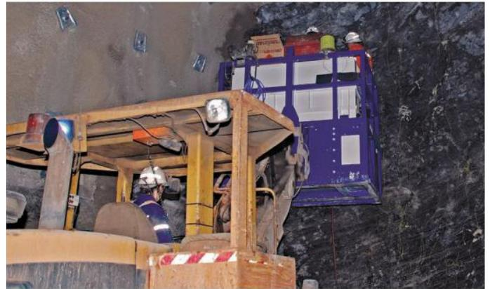
Improved lifter performance reduced the number of lifters and knee holes by four and a further three easer holes were removed from the standard ANFO pattern. The unit also recorded perimeter performance with string loading equivalent to that of packaged tube-type perimeter products.
