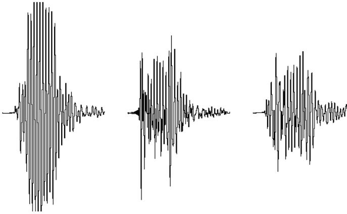
A single waveform is “stacked up” using different timing variables to simulate specific blast parameters.
