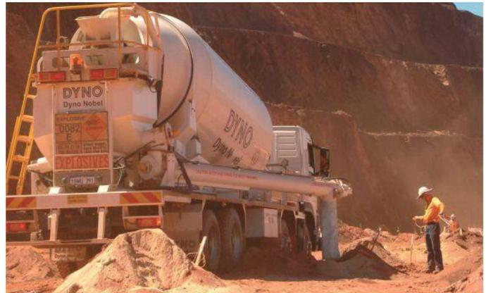
Reactive ground conditions, on the other hand, require special, approved explosives that inhibit the reaction between the pyritic ground and ammonium nitrate.
